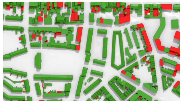
Figure 11: A common error we have noticed is the wrong orientation of semantic surfaces stored in MultiSurface . In this example, the correctly oriented RoofSurfaces are shown in green, and those with the inverted orientation (errors) are shown in red.
