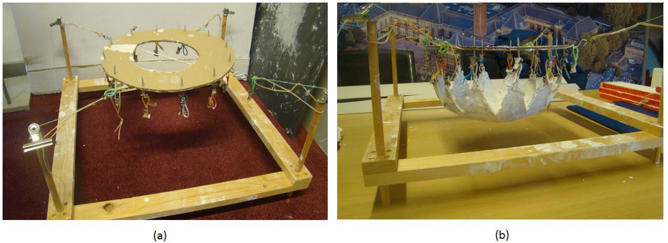
Figure 5-4: Supporting framework for the hanging model
