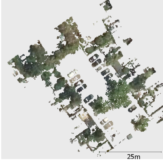
(a) Top view AHN4 class 1 points before height-based filtering
