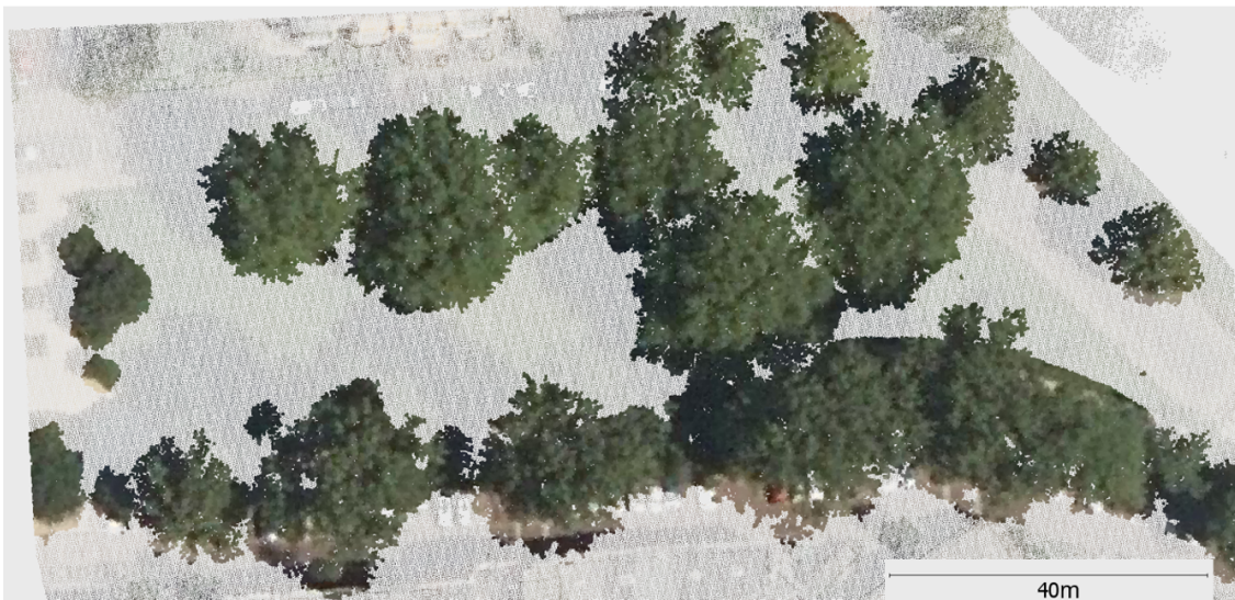
Figure A4: AHN4 colorized images from aerial imagery, larger points showing points above 2m and smaller points showing points below 2m.
