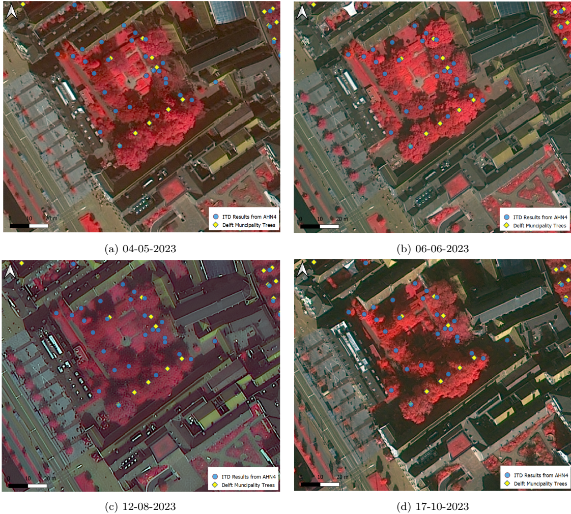
Figure 6.36: Four images showing the NDVI variation between late spring, summer and beginning of fall in 2023.
