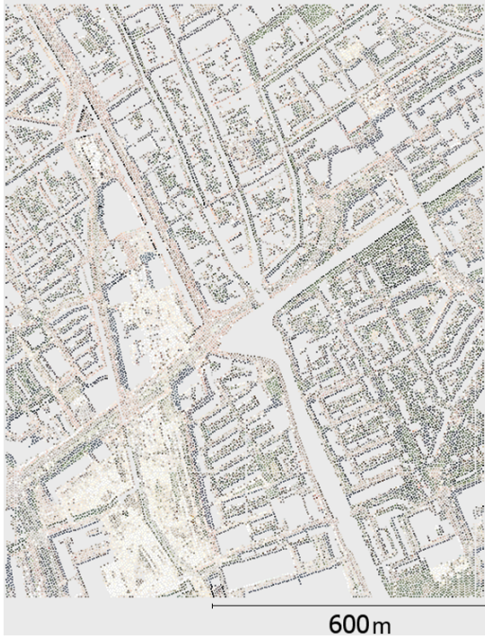
Figure 5.3: AHN4 class 2 ground points subsampled with a min distance of 5m
