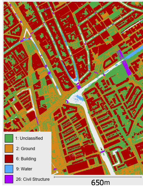
Figure 4.4: AHN classified tile (37EN1) 1x1.25km in Delft with classes based on Table 4.3
