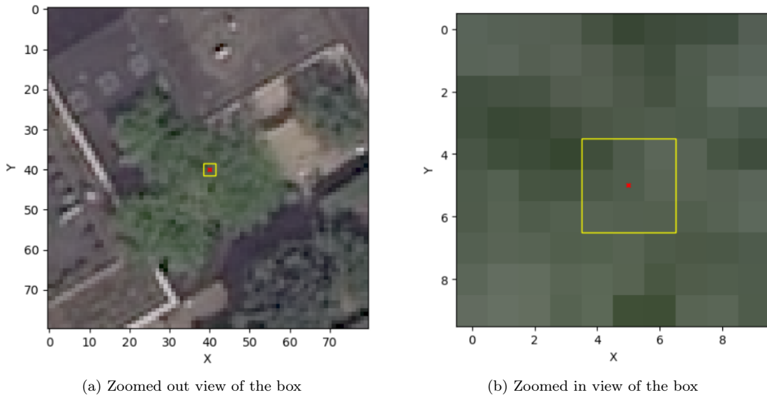
Figure 5.12: Spectral data extraction for tree location. The tree location is marked in red, and the mean RGB values are extracted within the yellow box, 0.9x0.9cm (Note that the axis is in pixel number, where one pixel is 0.3x0.3 cm).
