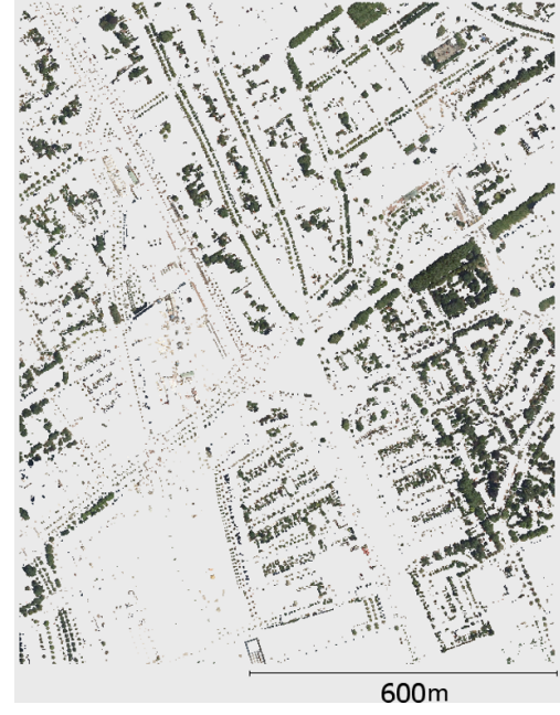
Figure 5.7: AHN4 class 1 in RGB after filtering points by 2 ground height
