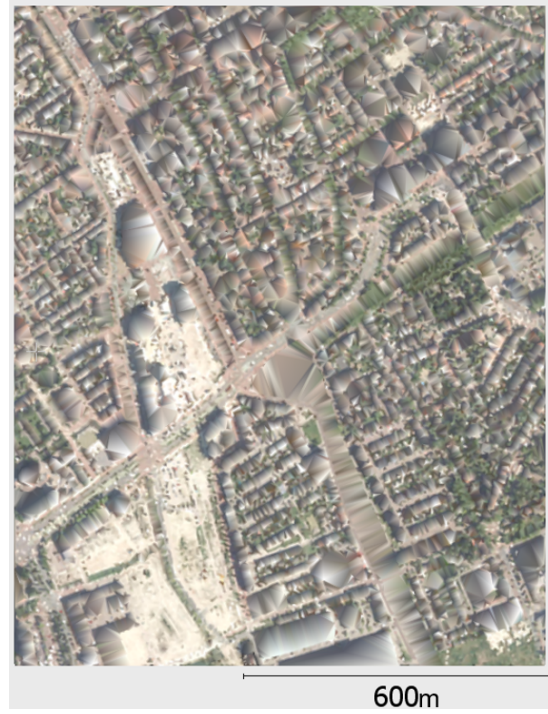
Figure 5.4: Intensity mesh of AHN4 class 2 ground points subsampled with a min distance of 5m
