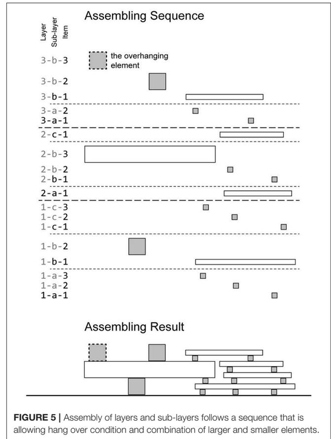
to ensure that the assembly is balanced at any moment during the construction phase. Moreover, the collision between the moving element on the gripper and the previously stacked elements is prevented.
