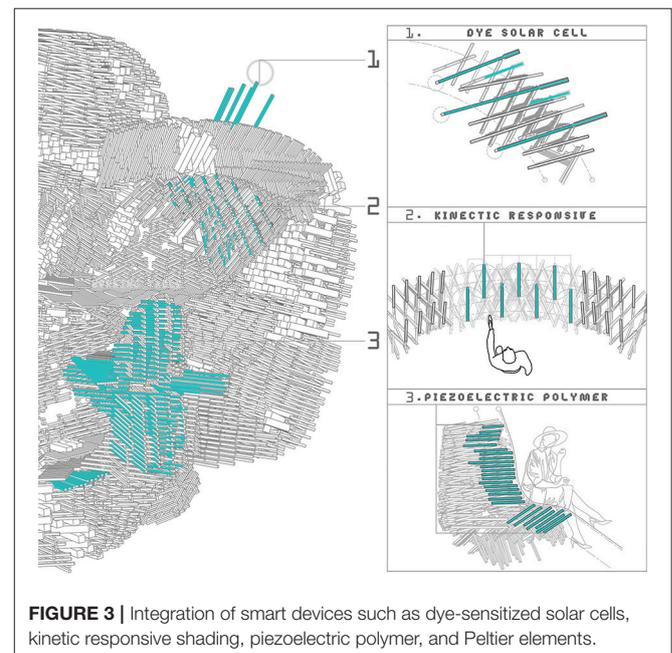
**FIGURE 3** | Integration of smart devices such as dye-sensitized solar cells, kinetic responsive shading, piezoelectric polymer, and Peltier elements.
