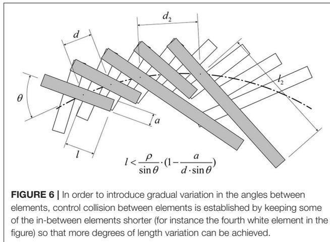
of elements is limited when the orientation of elements is not parallel to each other and the limit of the length is identified with an adjusted distance ( $d_2$ , shown in **Figure 6**).
