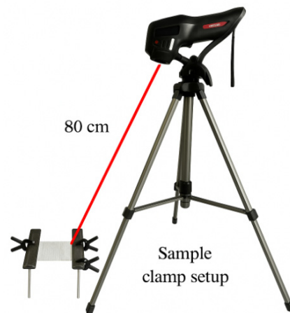
Figure 3. Experimental setup for thermal imaging measurements. A FLIR infrared camera is mounted on a tripod at a fixed distance of 80 cm from the sample, which is secured using a custom clamp to ensure stability during imaging.
