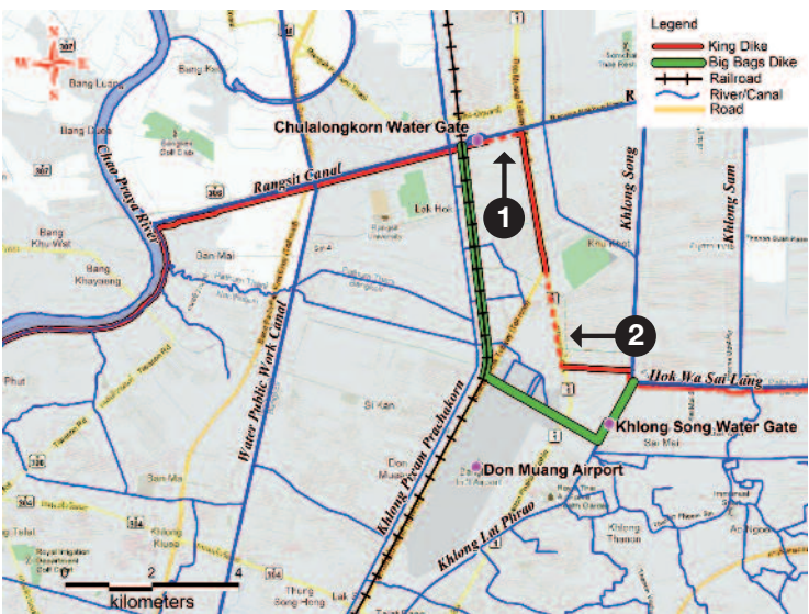
Figure 3.16 Openings (1 and 2) in the King’s dyke on the Northern side of Bangkok and the temporary dyke of big bags
