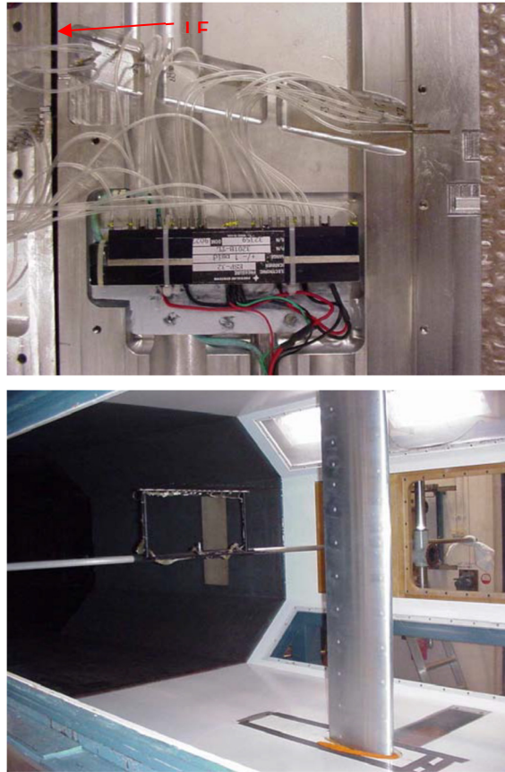
Figure 7.13 One of the sensors inside the 0.25 m chord DU91-model (with the lower side removed, leading edge at the left) and the test setup of the complete model in the test section, Boorsma (2003)
