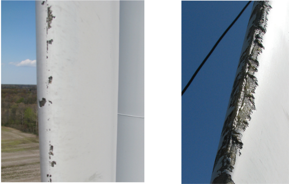
Figure 4.32 Leading edge erosion in various stages (Rempel 2012)
