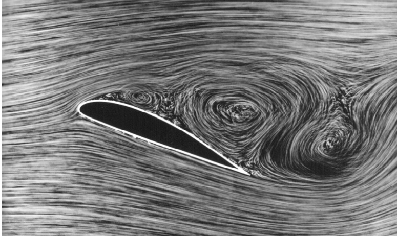
Figure PII-2: Flow visualization of an airfoil at about 20^\circ incidence showing leading edge separation. Photo DLR-CC BY 3.0 (Wikimedia Commons)
