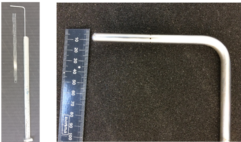
Figure 3.20: the Casella pitot-static tube used for test section dynamic pressure calibration curves.
