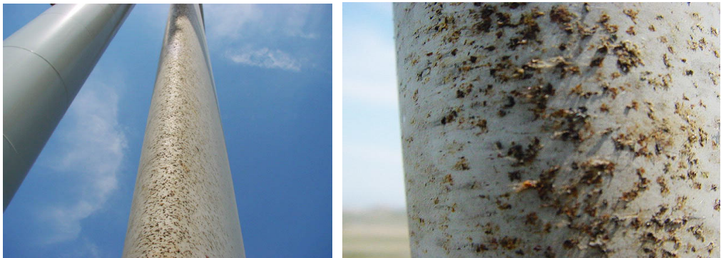
Figure 4.8: Insect debris on blades of turbines in the Magallon wind farm, Spain (Bladecleaning, 2005)
