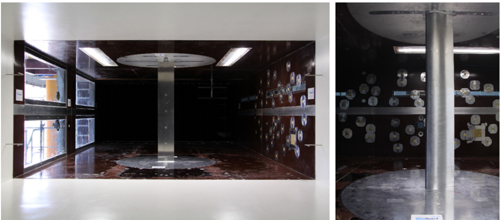
Fig. B1: The 1.25 \times 2.75 \text{ m}^2 test section of the DWG, showing a flat plate attached to the balance system under 90^\circ incidence (left) and a 0.2m model (right). Courtesy DWG
