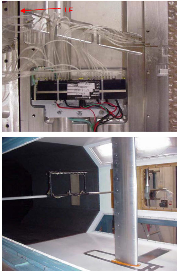
Figure 7.13 One of the sensors inside the 0.25 m chord DU91-model (with the lower side removed, leading edge at the left) and the test setup of the complete model in the test section, Boorsma (2003)
