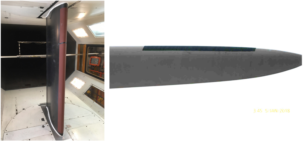
Figure 4.27: The test setup in the Delft LTT (left) and the test turbine blade with the sand paper installed. Right photo by I. Alting (ECN).
