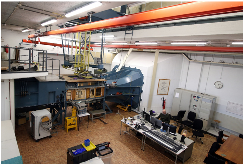
Figure 3.17: View on the LTT-test section, with in the middle the contraction. Also visible the overhead balance system. (Photo Henk Jan Siemer)
