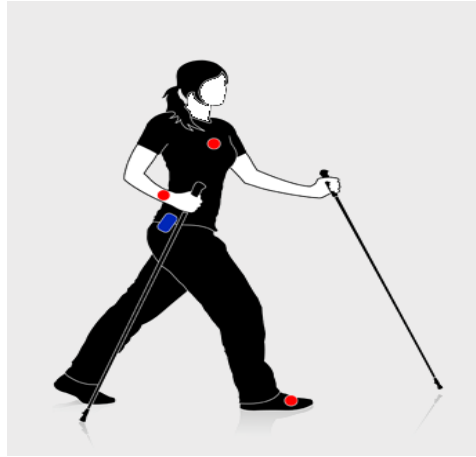
Figure 4.9: Placement of the three IMUs and the data collection unit [109].
