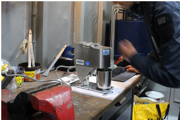
Figure 5.5: Usage of Fann 286 on board during the first time. Inside the cup is a BOB-geometry.
