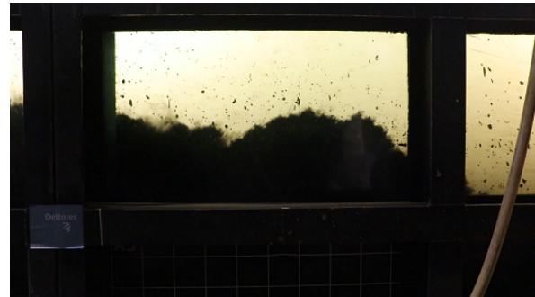
(d) Snapshot (2) of video recording: run 1, test 6. p_j = 1.00 bar, I_j = 401.6 N/m and SOD_r = 300 mm.
