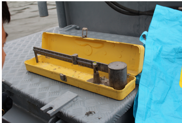
Figure 5.6: A mud balance to obtain a rough estimate of the density of a material, in this case harbour mud.
