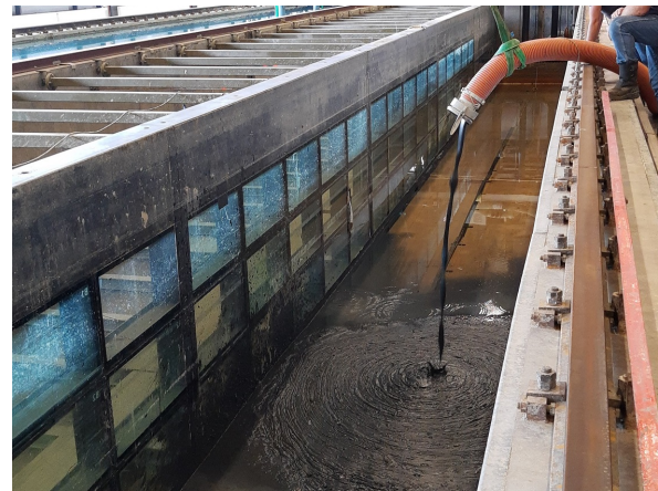
(d) Pumping the mud from the truck into the flume.
