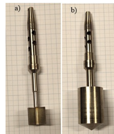
Figure 5.20: a) vane and b) bob geometry for the HAAKE™ MARS™ Rheometer (Goda, 2021)
