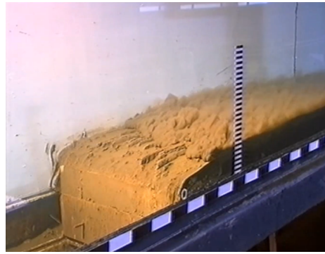
Figure 4.4: WID demonstration in a small scale flume at Deltares (Mastbergen, 1995).
