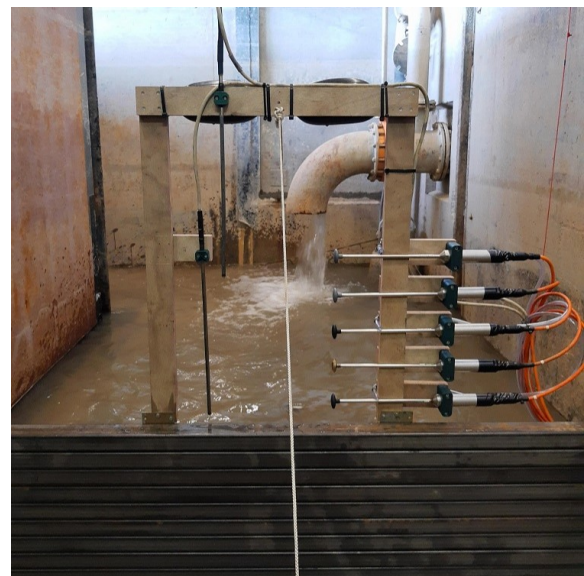
Figure 5.14: Photo of the measuring frame at the end of the flume.
