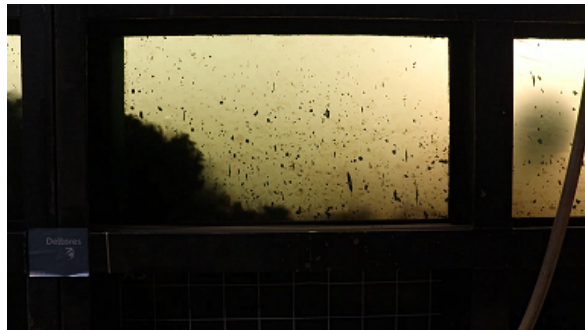
(c) Snapshot (1) of video recording: run 1, test 6. p_j = 1.00 bar, I_j = 401.6 N/m and SOD_r = 300 mm. Jetbar is still visible on the right side.
