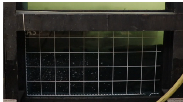
(b) Snapshot (2) of video recording: run 2, trial week. p_j = 1.07 bar, I_j = 426 N/m and SOD_r = 0 mm.
