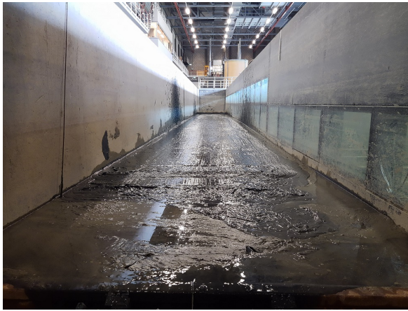
Figure 5.2: Impression of the flume after preparation of the sediment before the start of a test.
