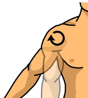
Facilitate arm movement with a moment of 0.95Nm at shoulder
