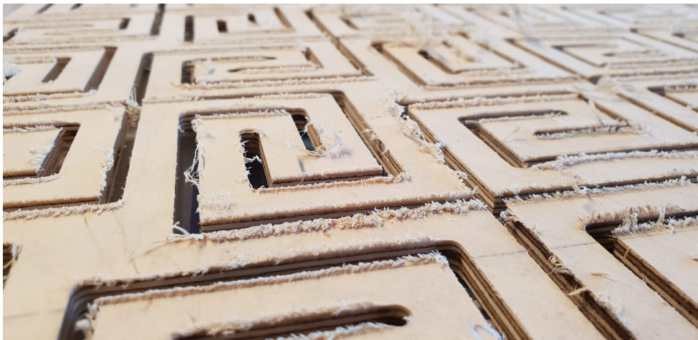
Figure 82. Close-up from the constructed panel, directly coming from the milling machine.
