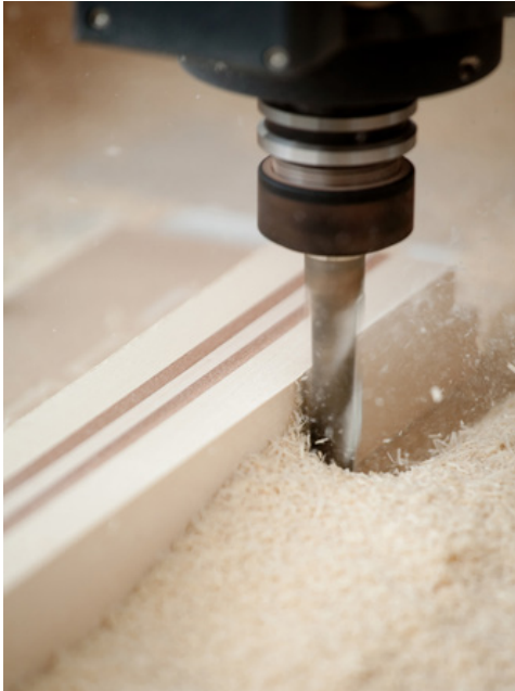
Figure 14. Cutting wood with a CNC milling machine (Niewegłowski).
