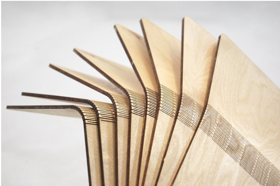
Figure 4. Linear pattern allows for flexibility in one direction (Couden, 2013).
