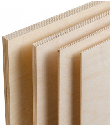
Figure 8. Plywood is constructed of multiple layers of wood veneer, giving it isotropic properties (US Craft Company, Unknown).
