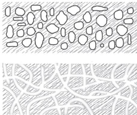
Figure 54. Schematic representation of closed (top) and open (bottom) pore structures (adapted from Cremer and Muller (1982) ).
