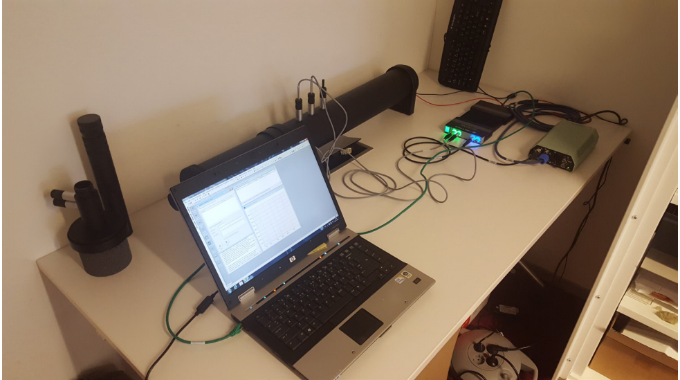
Figure 62. Setup for Impedance Tube measurement.
