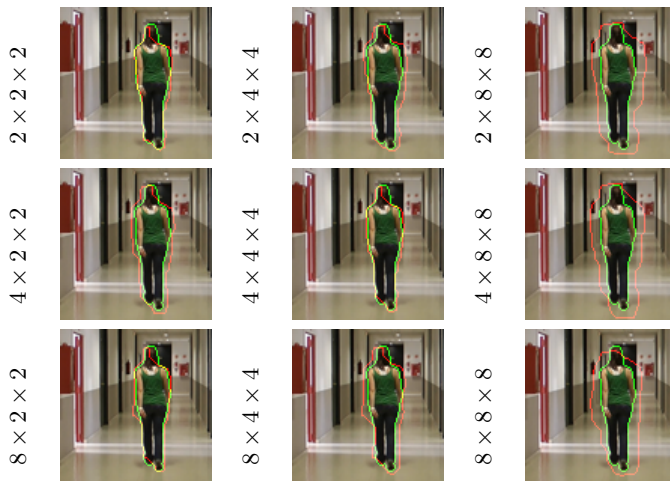
Fig. 13: Qualitative comparison of the different patch sizes for I\_BS\_01 sequence of LASIESTA dataset, green contour: ground truth and red contour: the output of the method.
