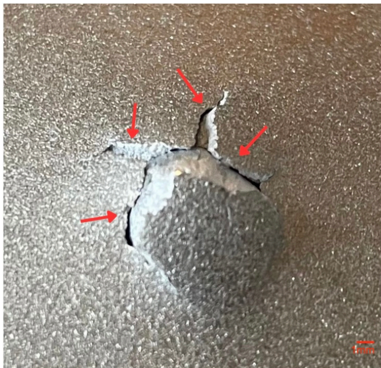
Figure 5.39: Four-split crack in the back of substrate MPAir 140J
