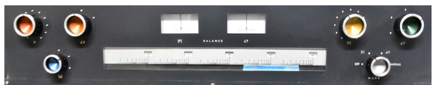
Figure 6. The null-meters, the s-scale and various controls
