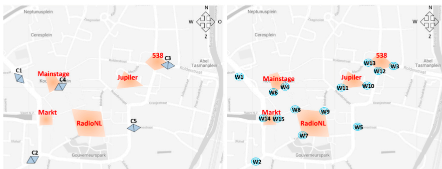
Figure 2. The layout of the sensor network depicted on a map for the TT Festival terrain of 2018, where the circles with the W-code represent the Wi-Fi sensors and the double triangles with the C-code represent the automated counting systems.
