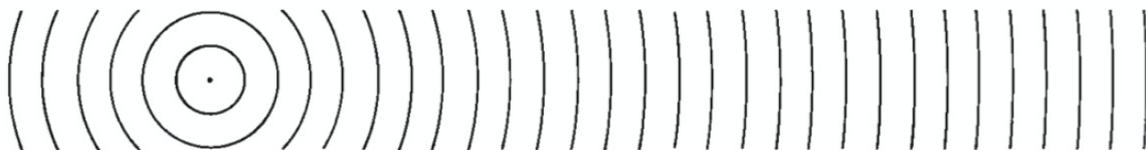
Figure 1.3: The flattening of spherical waves with distance [4]
