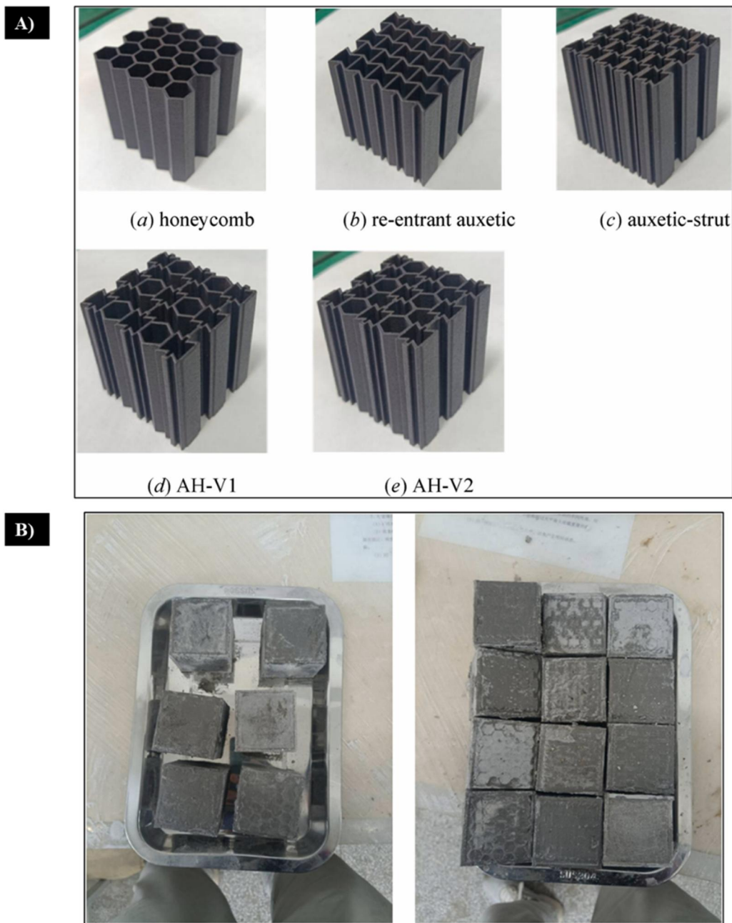
Figure 28. (A) The cellular structures made from 3D-printed PA6 and (B) the concrete specimens at the stage when the mold is prepared for removal [404].
