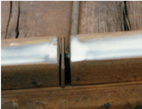
Figure 1.7: Debonding of end post layer [13]
