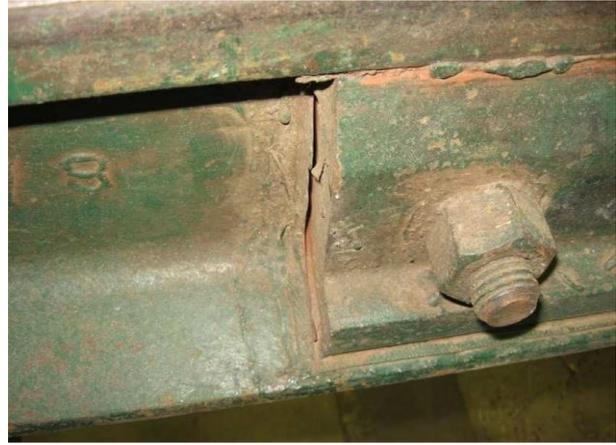
Figure 1.6: Debonding of the insulation layer [7]
