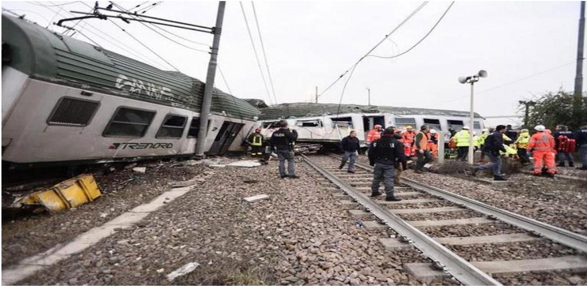
*Figure 1.11: Derailment accident due to malfunction of an IRJ, January 2018, Milan [15]*
