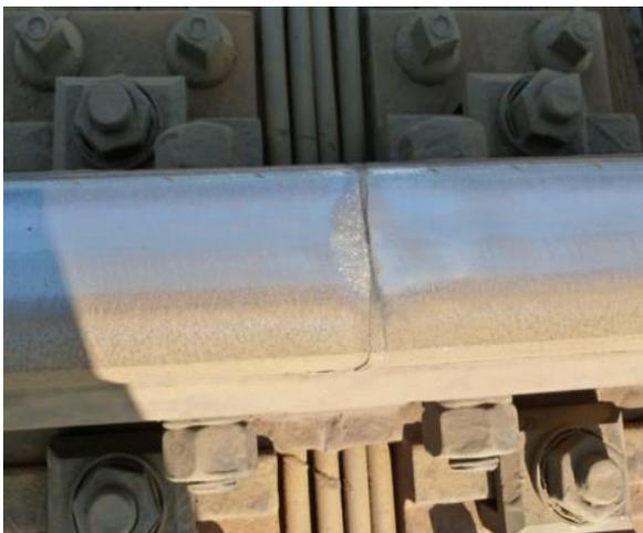
Figure 1.9: Crushed end post and metal flow [13]
