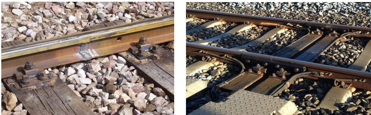
Figure 1.1: a) welded connection [1] b) jointed connection
