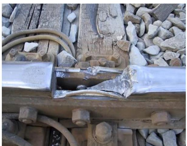
Figure 1.8: Broken rail in the vicinity of IRJ [13]
