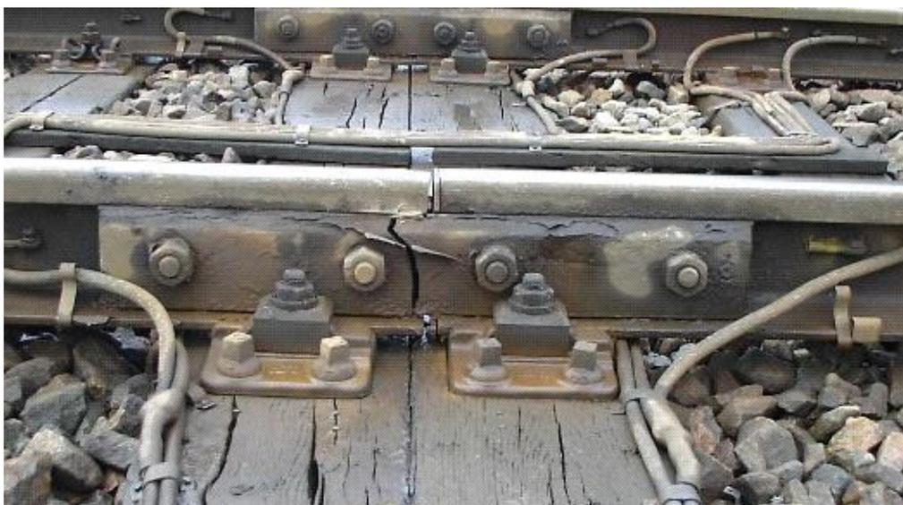
Figure 1.5: Broken fishplate [13]
