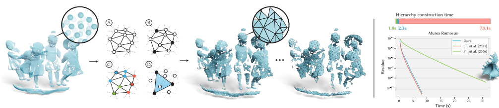
Figure 4.1: Illustration of our hierarchy construction for one level. Starting from a mesh or point cloud, A) we construct a neighbor graph on the surface. B) We then sample a spatially uniform set of nodes, C) compute the graph Voronoi diagram of the samples, and D) project unsampled points onto triangles formed by edges between Voronoi neighbors. This is repeated for every level. Right: Comparison of run time for solving a Laplace system on a triangle mesh. Our hierarchy construction is fast, while achieving similar solver performance to the state-of-the-art.
