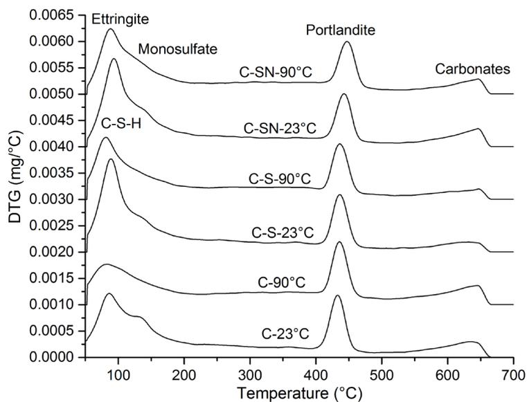
**Figure 5: DTG curves of 30 days old cement pastes**
