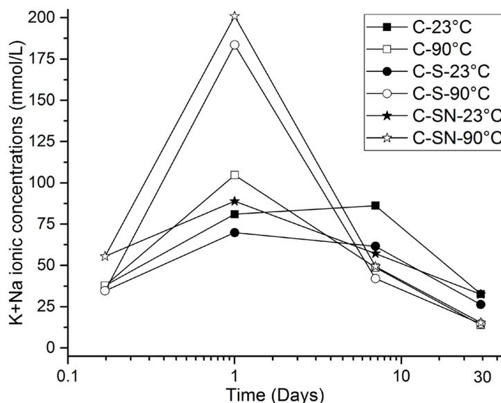
**Figure 7: Pore solution k+Na concentration at different ages**
