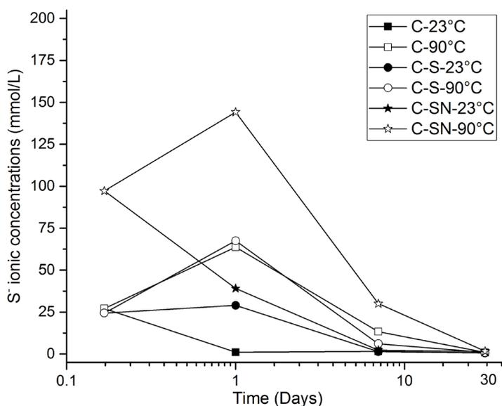
**Figure 6: Pore solution S<sup>-</sup> ion concentration at different ages**
