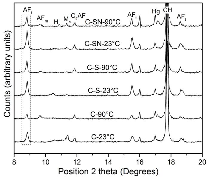
**Figure 4: XRD patterns of 30 days old cement pastes**
