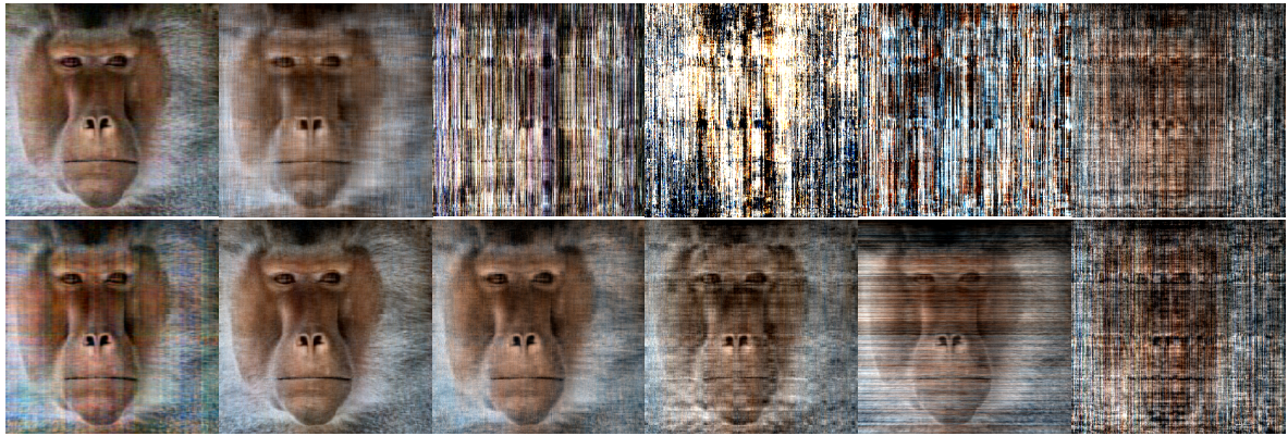
Figure 4-2: Effect of varying CP Rank on Image Reconstruction with kNN = [1 1 1]. Top Row: \lambda_l = 0 , Bottom Row: \lambda_l = 0.001 , Left to Right: CP Rank R = [20\ 40\ 60\ 80\ 100\ 120\ 140]
