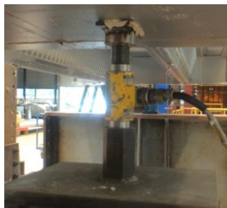
a) Load cell, connected to the computer and placed underneath the specimen
