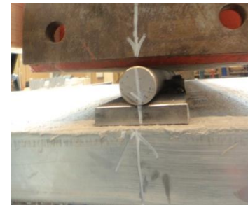
c) Steel strip plus rod in between the test specimen and the steel beams.
