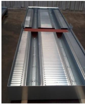
a) ComFlor210 specimen including the joist shuttering, ready to place the reinforcement.
