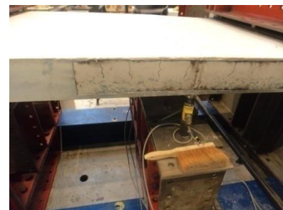
Figure H 28 Crack pattern of the fourth specimen. Failure at 665 mm away from the point of engagement of the load, right above the support B. Crack pattern can be seen on the side of the specimen.
