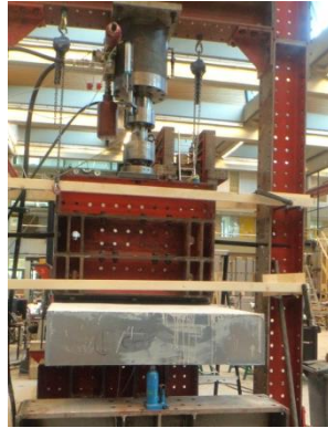
a) Overview portal with the hydraulic cylinder.
