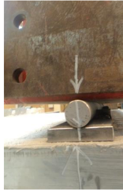
b) Point of engagement on the specimen, allowing rotation.
