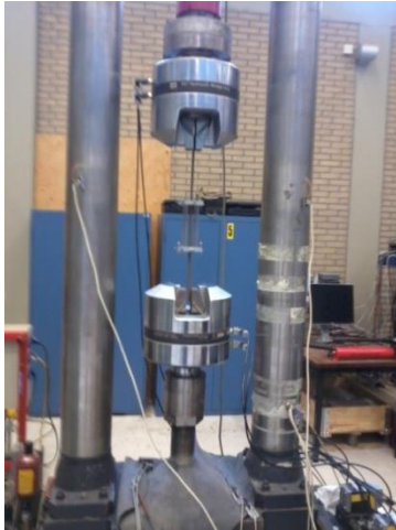
a) Test rig before testing the individual reinforcement bars
