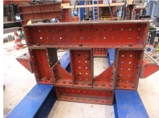
b) Mechano parts to serve as a temporary support at the right height before testing, connected to the underlying steel beams.
