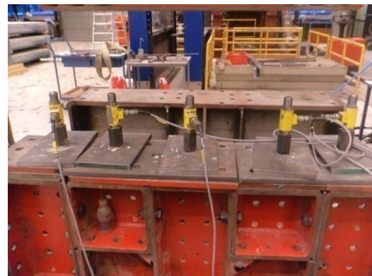
b) Support B, ComFlor75 setup. Five load cells to support 5 ribs.
