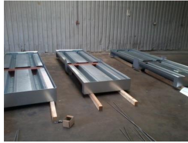
b) All three ComFlor210 specimens in place, including the integrated HE200A steel beam.
