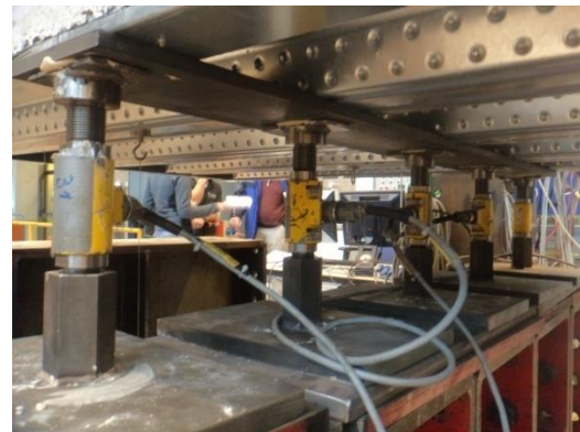
b) Final mid support of the ComFlor75, test specimen 5, in place.
