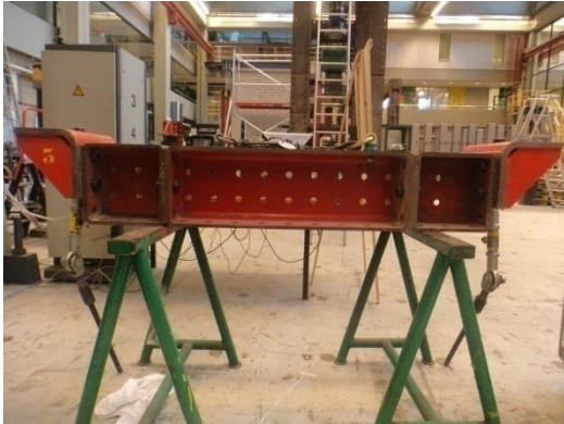
a) Beam that will be placed on top of the specimen, to serve as a support
