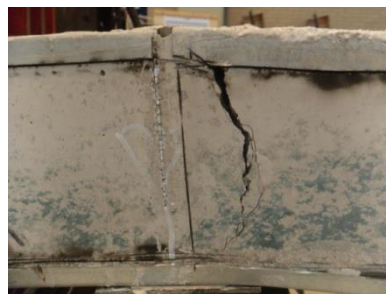
Figure H 28 Crack pattern of the fourth specimen. Failure at 665 mm away from the point of engagement of the load, right above the support B. Crack pattern can be seen on the side of the specimen.
