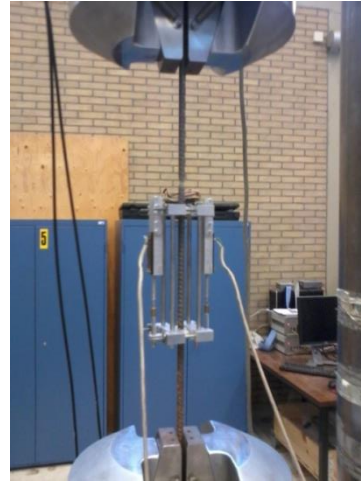
b) Reinforcement bar at the moment of failure.
