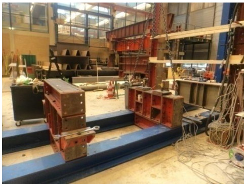
a) Base parts of the test rig on top of the two main beams that transfer the forces to the floor.
