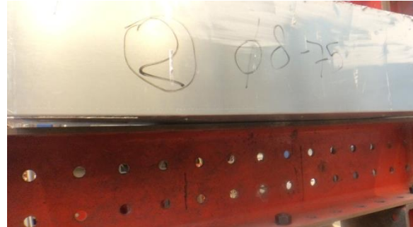
b) Specimen at the start of the test. It has been lifted a little bit to avoid resistance to rotations of the specimen.
