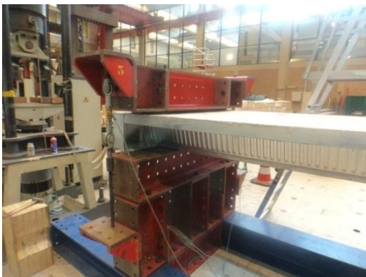
a) Final end support detail with a ComFlor210 specimen in place.
