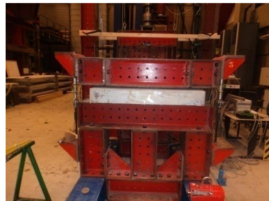
b) Final end support detail with a ComFlor75 specimen in place.
