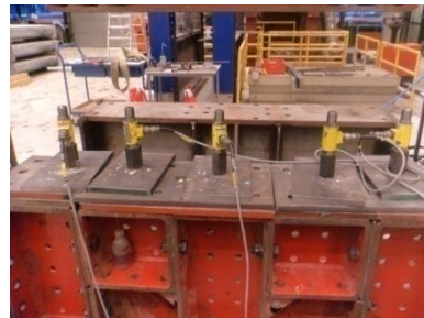
b) All five load cells before placement of the specimen on top.
