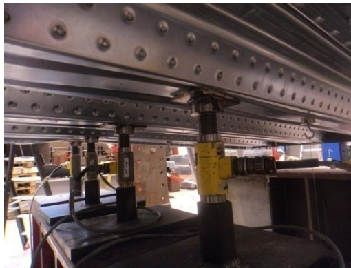
Figure 7.2 Punching shear above each load cell (inward buckling of the ComFlor75 sheet)
