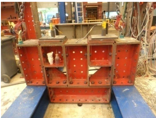
a) Support B, ComFlor210 setup. Two load cells to support both ribs.
