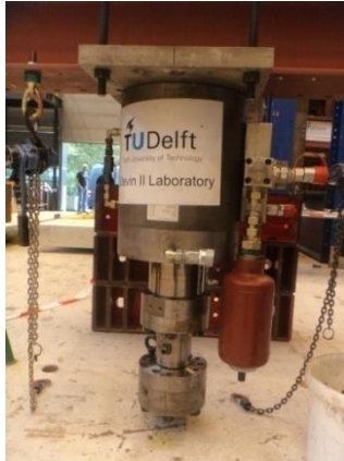
a) The hydraulic cylinder used to apply the force.
