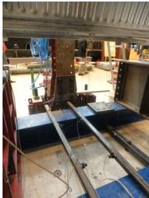
a) Overview of the four applied thread-LVDT's under the specimen.
