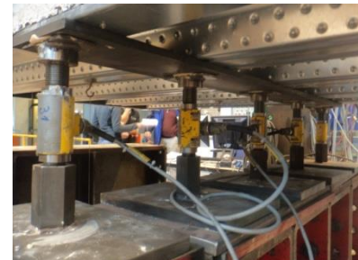
c) All five load cells including the steel strip underneath the last specimen.
