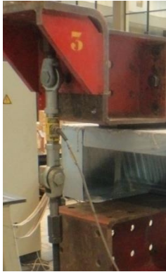
a) Load cell in tension
