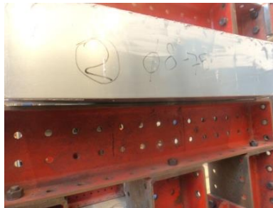
a) Lifting the specimen at the beginning of each test to assure free rotation
