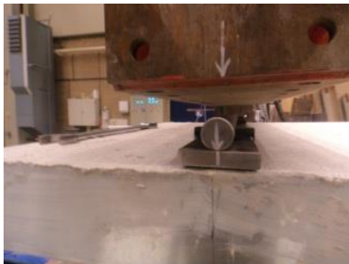
Assuring exact positioning of the applied load
