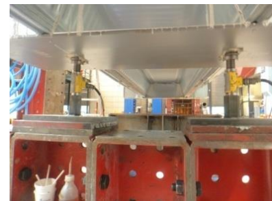
b) Overview of both load cells underneath the integrated steel HE200A beam.
