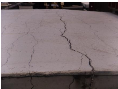
Figure H 28 Crack pattern of the fourth specimen. Failure at 665 mm away from the point of engagement of the load, right above the support B. Crack pattern can be seen on the side of the specimen.
