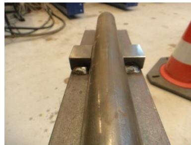
b) Horizontal displacement restrictions.
