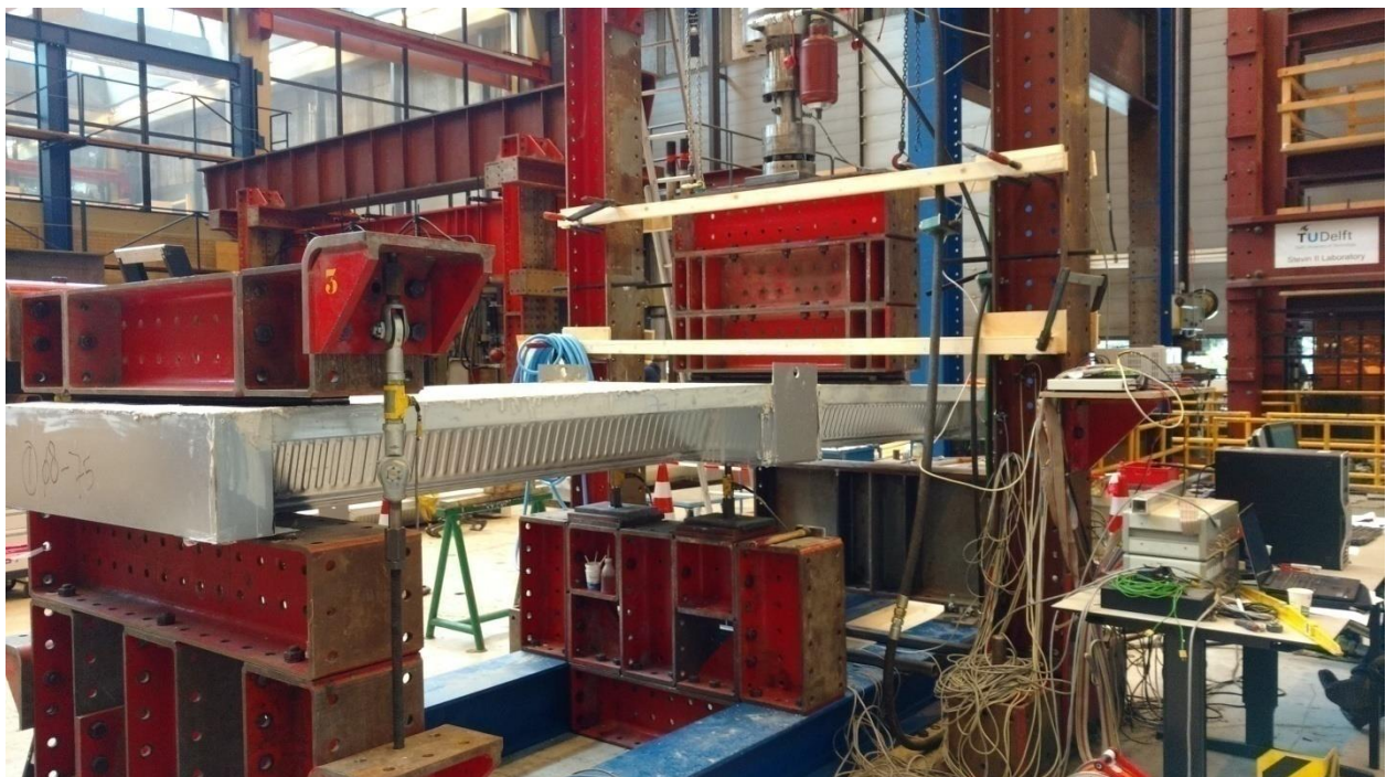
Figure 6.2 Overview test setup for one of the ComFlor210 specimens.
