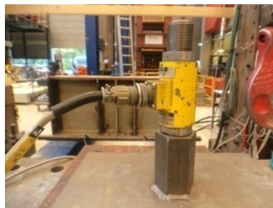
a) Load cell before placement of the specimen.
