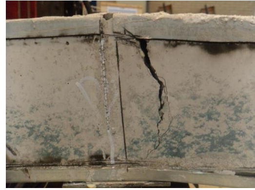
b) Moment of failure, the joist shutterings at the bottom could contribute slightly as well as the strips on top that connect the joist shuttering to the ComFlor75 sheet.
