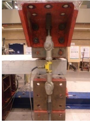
b) Load cell in tension ComFlor75
