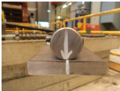
a) Steel strip with a rod on top to create a hinge.
