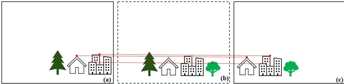
Figure 9: The in-between image(b) is generated by interpolating the left image(a) and the right image(c), using the red tie-points.
