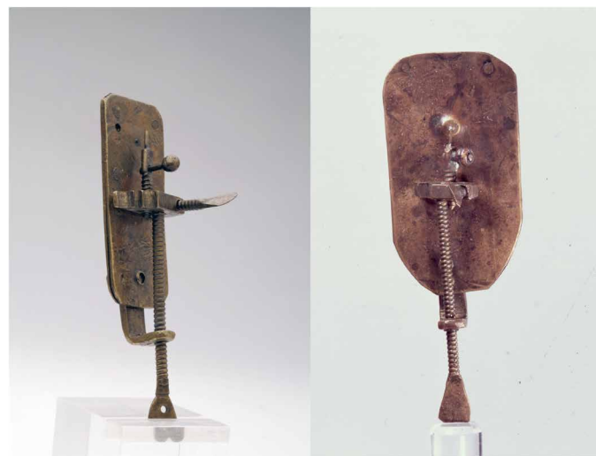
Fig. 1. The two original Van Leeuwenhoek microscopes that were studied with neutron tomography. The lens sits mounted between the brass plates, at the position of the specimen pin. (A) A medium-powered ( \times 118 ) instrument (Rijksmuseum Boerhaave, Leiden, inventory number V7017). Note that there is a redundant drill hole in the upper left corner of the instrument, not to be confused with its lens aperture, which is directly behind the pin. This microscope is numbered #1 by Van Zuylen. Photo credit: Tom Haartsen Fotografie, Ouderkerk aan de Amstel. (B) The instrument with the highest magnification among the preserved ones ( \times 266 ) (Utrecht University Museum, inventory number UM-1). This microscope is numbered #3 by Van Zuylen. Photo credit: Utrecht University Museum.
