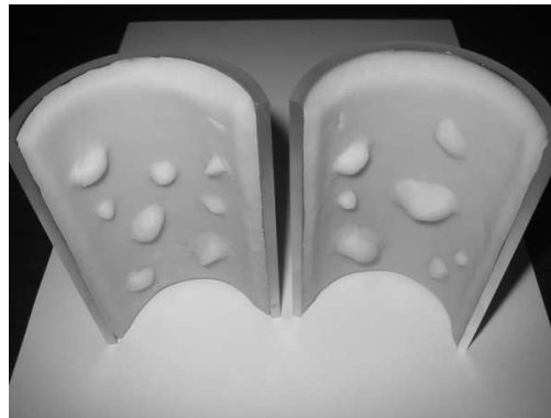
Figure 6.1: Phantom colon with plasticine objects. Photograph shows two halves of a cylinder inserted into a tight-fit second cylinder before scanning.
