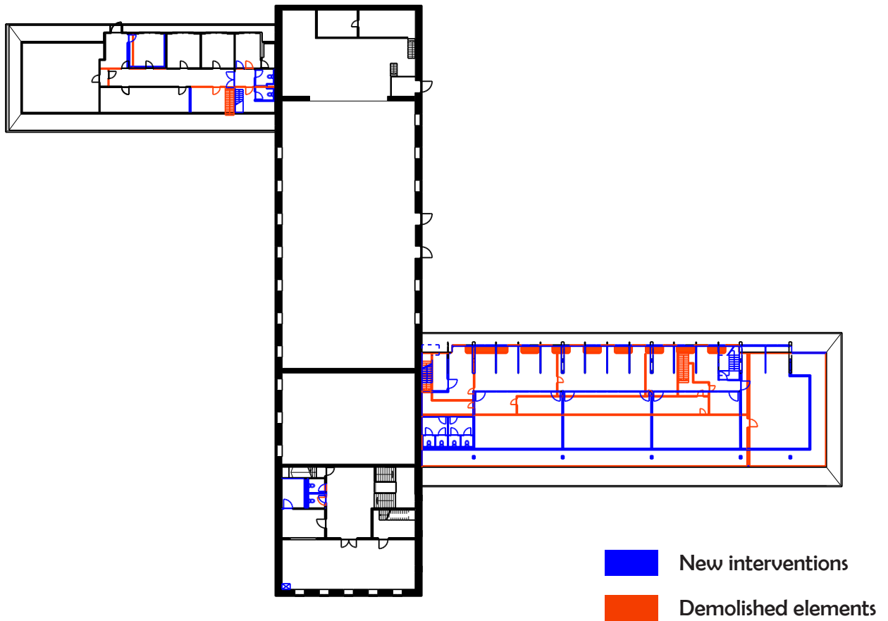
Demolition plan first floor 1:600
