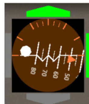
Figure 4.7: Roll and pitch indicators commanding a right bank and pull up (Maertens, 2009)
