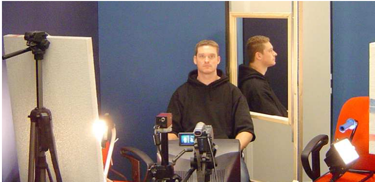
Figure 4.2: The physical settings for the case when the side view of the speaker's face was obtained by means of a 45^\circ placed mirror.
