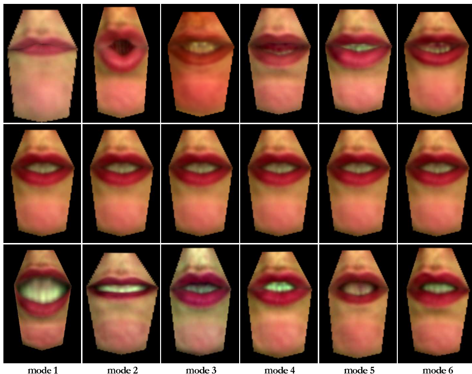
Figure 6.3: Combined shape and appearance statistical model. The images show from left to right the first six most important components in PCA terminology. These modes account for 78.65% of the total variation. Centre row: Mean shape and appearance. Top row: Mean shape and appearance +2\sigma . Bottom row: Mean shape and appearance -2\sigma .
