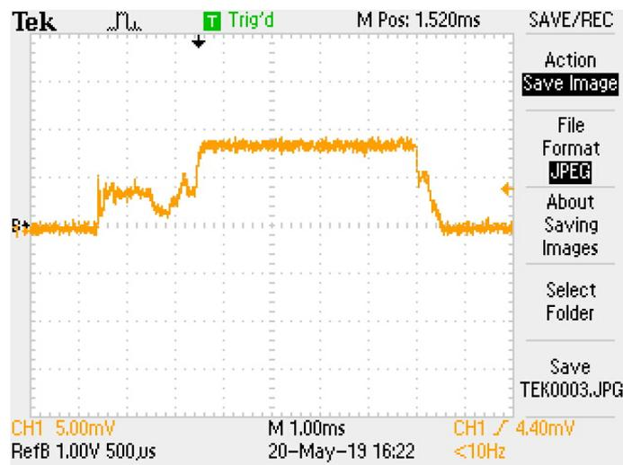
Figure 6.3: Current measurement sending 100 Byte
