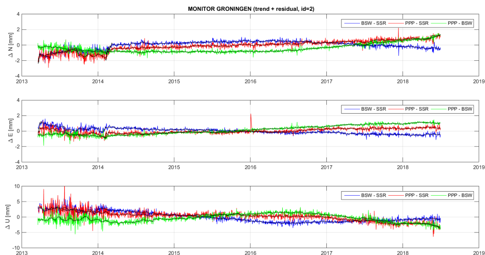
Figure 6.5: Trend differences for the Groningen monitoring stations for all combinations: SUM_TREND+RESIDUAL_GRO . The colored lines are time series of daily averages for the different combinations, the black lines are the moving 21 day median of the daily averages (with outlier and step detection).
