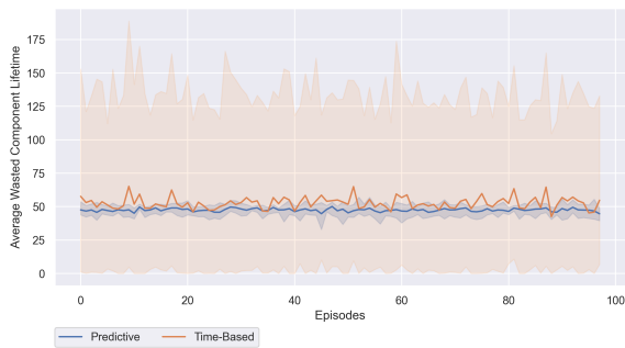
Figure 3.13: Average wasted component lifetime for several T_a values, indicating the ( Min-Max ) values.
