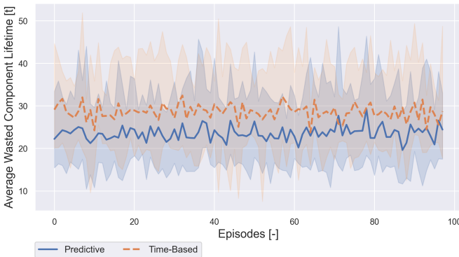
Fig. 37: Scenario 2: Average wasted component lifetime for N_e = 100 and N_s = 10 during testing. Note: CM and IM are omitted because the values for all episodes would be 0 and 1 respectively.
