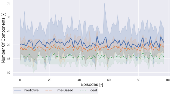
Fig. 30: Scenario 1: Number of components for N_e = 100 and N_s = 10 during testing. Note: CM is omitted because it has the same values as the IM policy.
