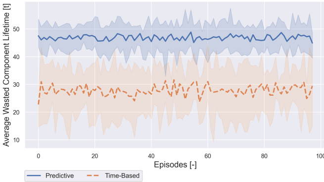
Fig. 31: Scenario 1: Average wasted component lifetime for N_e = 100 and N_s = 10 during testing. Note: CM and IM are omitted because the values for all episodes would be 0 and 1 respectively.
