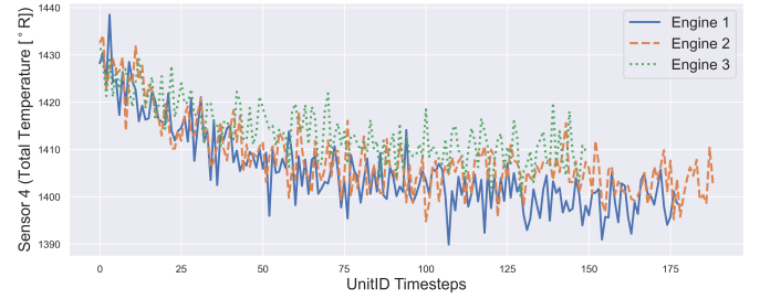
Fig. 7: Overview of Sensor 4 for three arbitrary engines of subset FD001 (C-MAPSS Dataset).
