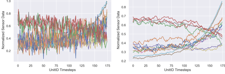
Fig. 8: The influence of exponential smoothing on sensor data from one specific engine. In the left graph \alpha_s = 0.9 was used, in the right graph \alpha_s = 0.1 .
