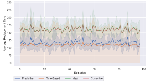
Figure 3.14: Average replacement lifetime for several T_a values, indicating the ( Min-Max ) values.
