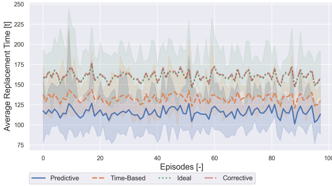
Fig. 33: Scenario 1: Average replacement time for N_e = 100 and N_s = 10 during testing.
