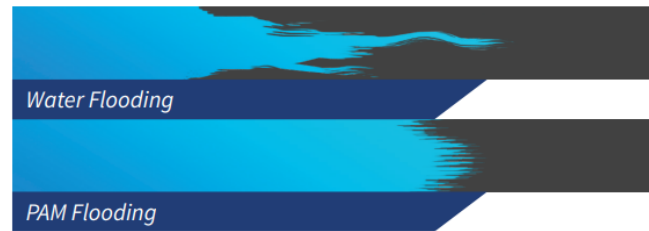
Figure 2.2: Stabilised front by the addition of polyacrylamide to the drive water [12].
