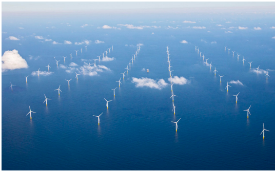
(a) Aerial view of offshore wind farm Gemini, where the turbines are still placed in a grid-like layout, retrieved from [115].
