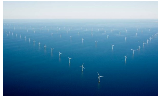
(b) Aerial view of offshore wind farm Kriegers Flak, where optimisation caused an asymmetrical layout, retrieved from [26].
