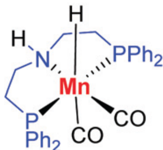
Figure 1.2: Manganese-based metal complex surrounded by PNP-pincer complex and auxiliary ligands[19]
