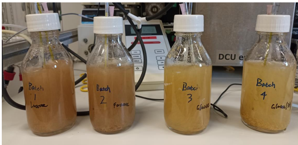
Figure 3-5 Setup of the batch test with 4 bottles (from left to right: lactate dosing; formate dosing; glucose dosing; glucose dosing with 3-hour anaerobic time)
