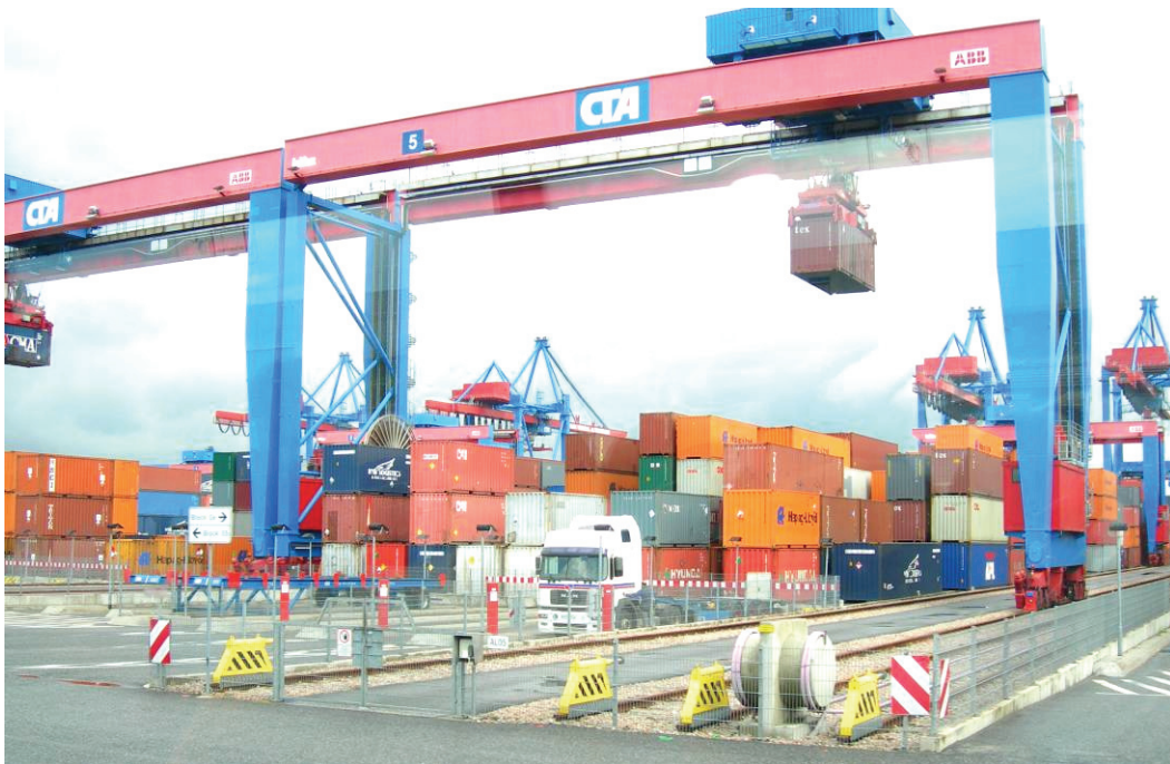
Figure 5.21 Automated RMG performing landside transfers at CTA, Hamburg
