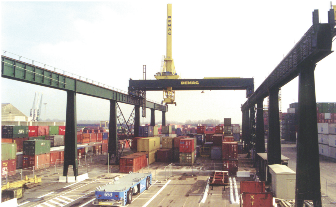
Figure 5.23 Discontinued test plant of an automated OBC, Hessenatie Antwerp (Gottwald)
