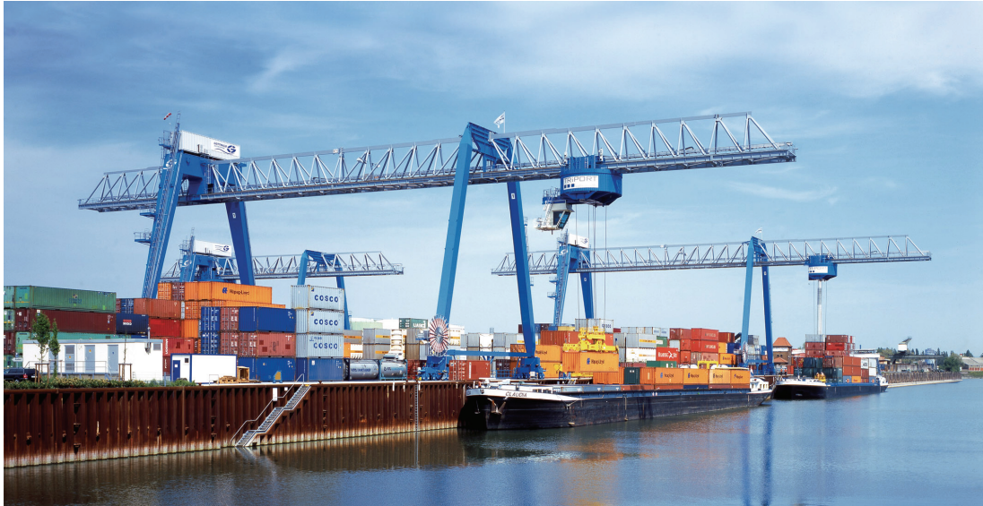
Figure 5.9 Wide-span gantry crane on inland terminal Ludwigshafen (Gottwald)
