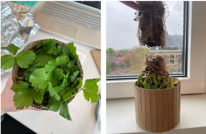
Figure 7.7: Main challenges in plant test samples preparation: left: altering the morphology of the plant and its leaves, right: minimizing the influence of roots on the experiment
