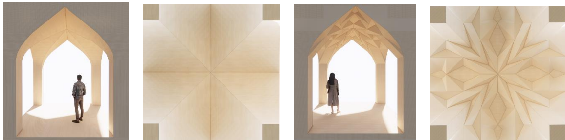
Figure 9: final possible spaces after shaping with predefined blocks (from left to right: (1) gothic vault , (2) gothic vault viewed from bottom, (3) diamond vault, (4) diamond vault viewed from bottom)
