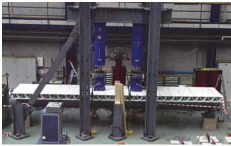
FIGURE 10: Four-point bending experiments on FRP-steel girder system [7].
