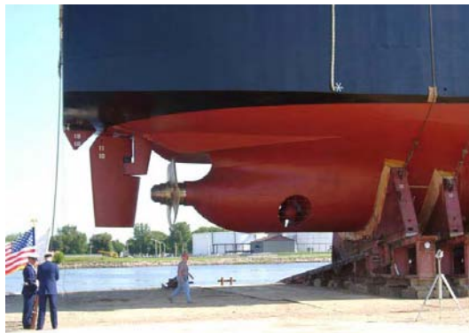
(d) The stern of a ship, showing the main propeller with the rudder and a tunnel thruster.
