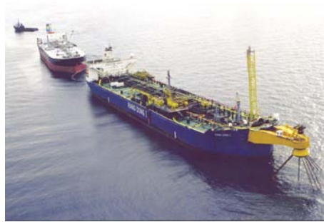
Figure 1.2: Example of spread turret mooring.
