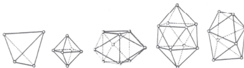
Figure 10: Dense Random Packing of hard spheres: polyhedra formed according to Bernal [44]
