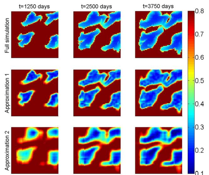
**Fig. 3** Oil-water front with tensor approximations. Approximation 1 has modal rank  $(20, 20, 5)$ . Approximation 2 has modal rank  $(10, 10, 5)$ . Colors represent oil saturation
