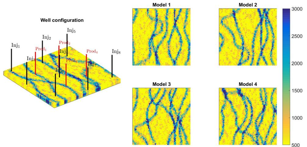
We have used a rectangular-shaped geometry instead of the egg-shaped reservoir described originally in [19]. The well configuration is composed of eight injectors and four producers. A view of some geological realizations is depicted in Fig. 6.
