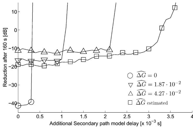
Fig. 2. Reduction of RPFxLMS after 160 s obtained for various choices of  $\widehat{\Delta G}$ , versus additional delay in  $\widehat{G}$ .
