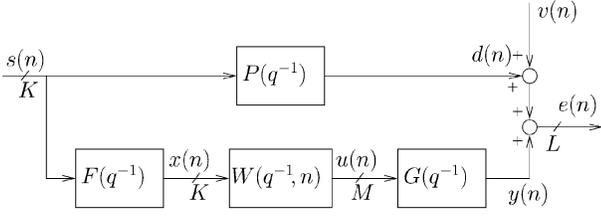
Fig. 1. Block scheme of the general multichannel feedforward active control system, with  $K$  reference,  $M$  control, and  $L$  residual signals.
