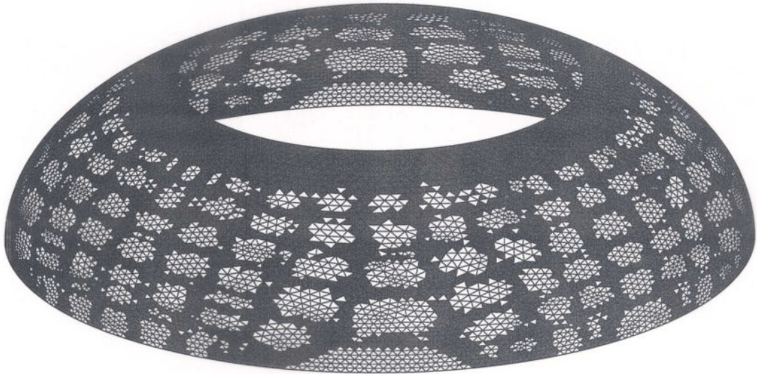
Figure 1.10 - Evolutionary Structural Optimisation of a shell structure by sequentially removing elements of low stress [13].
