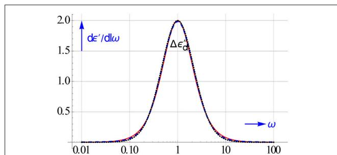
**FIGURE 19 | The KK conversion allows the calculation of  $d\varepsilon'/d\ln\omega$  from  $\varepsilon''$  data.** The figure compares the plain, direct  $\varepsilon''$  conversion of Equation (4.13) and the special one of Equation (7.8), by taking  $\varepsilon''$  data of a Debye relaxation polluted by conduction.
