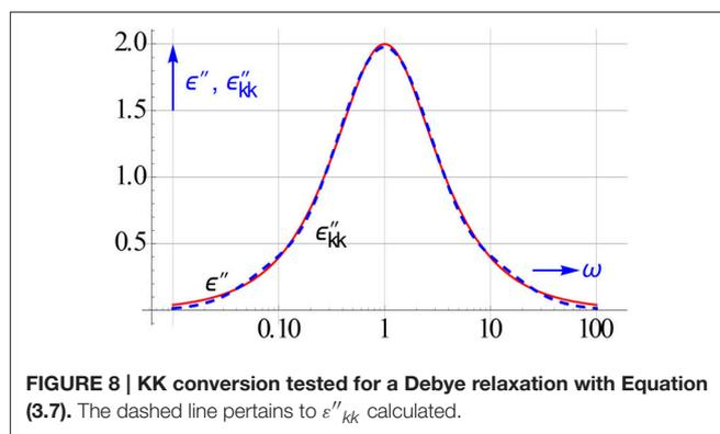
**FIGURE 8 |** KK conversion tested for a Debye relaxation with Equation (3.7). The dashed line pertains to  $\epsilon''_{kk}$  calculated.
