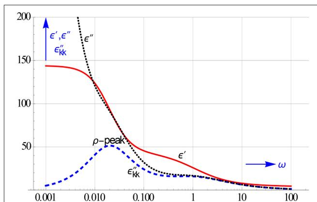
**FIGURE 3 | The l.f.  $\rho$  or space charge relaxation, which is due to the rather slow up and down motion of the ion clouds near the electrodes, remains hidden in the  $\epsilon''$  curve.** It too can be disentangled from the conduction contribution by calculating  $\epsilon''_{kk}$ . The conduction, which stems from the gross ion motion, appears alongside the EP, if the electrodes are not fully blocking.
