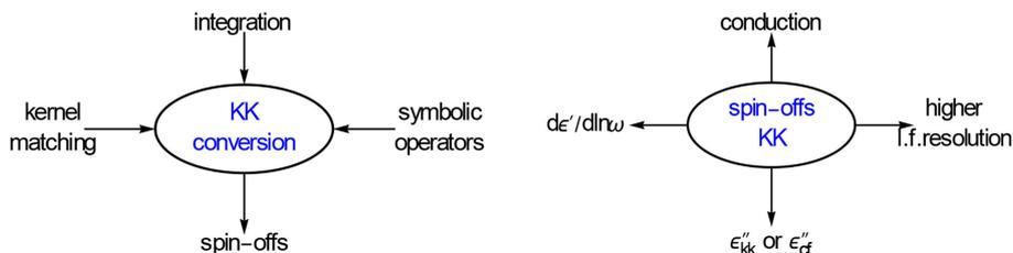
**FIGURE 5 | On the left, numerical integration is not the favorite tool for KK conversion.** It can be better realized with kernel matching and with symbolic differential operators. The conversion produces useful spin offs, they are depicted on the right. The higher resolution results from the elimination of the conduction from the  $\varepsilon''$ -data.
