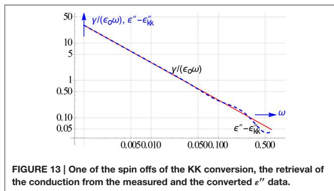
FIGURE 13 | One of the spin offs of the KK conversion, the retrieval of the conduction from the measured and the converted  $\varepsilon''$  data.
