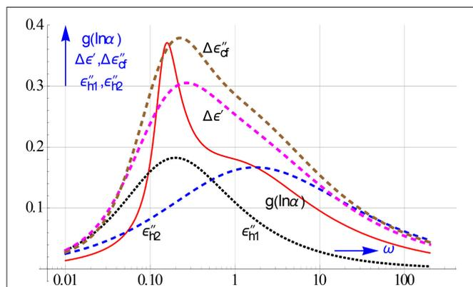
**FIGURE 20 | Evidence of the strong resolution power of the distribution function.** Using Equation (8.3) we computed the distribution from a rational all-in-1 modeling to  $\varepsilon'$  and  $\varepsilon''$  of the 2 overlapping HN relaxations employed before in **Figures 15, 18**. The underpinning relaxations can also be distinguished in the spectra of the differences  $\Delta\varepsilon'$  and  $\Delta\varepsilon''_{cf}$ , this is in particular true for the latter.
