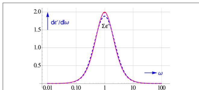
**FIGURE 10 | Accuracy of 3 options for computing  $d\varepsilon'/d\ln\omega$  for a Debye relaxation.** The commonly used central frame of Equation (3.11) is evidently not the best near the maximum for  $h = 2$ . The offset at the maximum disappears if we reduce  $h$  to  $10^{0.2}$ .
