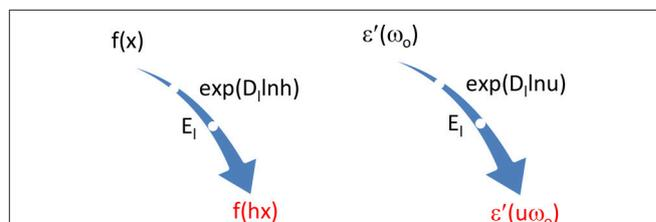
**FIGURE 11 | On the left, two symbolic tools to transform  $f(x)$  to  $f(hx)$ . On the right, trick to link  $\varepsilon'(u\omega_o)$  symbolically to  $\varepsilon'(\omega_o)$  and thus push the latter out of the convolution integral of KK in Equation (4.8).**
