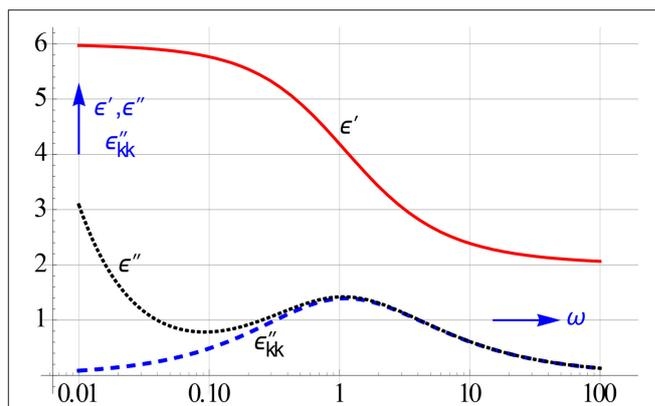
**FIGURE 1 | Simulated observed  $\varepsilon''$ -spectrum and that of  $\varepsilon''$  calculated by converting  $\varepsilon'$ -data into conduction free  $\varepsilon''$ -ones.** Only the latter shows us the authentic loss peak we look for. The  $\varepsilon'$ -spectrum remains unaffected by conduction. We assumed that the electrode polarization, which may also turn up at low frequencies, can be neglected, cf. **Figure 3**.
