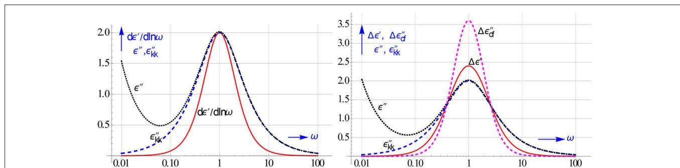
**FIGURE 17 | On the left peak shape of  $d\varepsilon'/d\ln\omega$  compared to that of  $\varepsilon''$ .** On the right the peaks of the logarithmic differences  $\Delta\varepsilon'$  and  $\Delta\varepsilon''_{cf}$ , in particular the latter is much spikier than  $\varepsilon''_{kk}$ . The curves are given for a Debye relaxation and  $h = 2$ . The rise in  $\varepsilon''$  in the low  $\omega$  region is caused by ohmic conduction, it clearly lessens the resolution.
