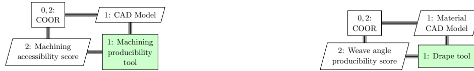
(a) XDSM visualization of the machining subworkflow (b) XDSM visualization of the stamp forming subworkflow
