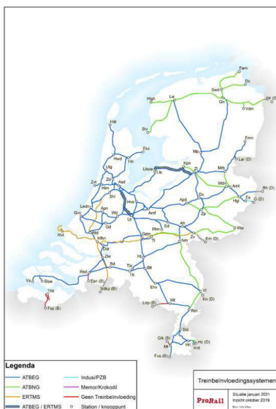
Figure 1.4: Coverage of Automatic Train Protection systems on the Dutch railway network.
