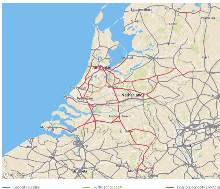
Figure 1.1: Overview of the Dutch railway network on a standard day in the 2026 timetable year. Source: Timetable Redesign: Capacity Model 2027, Netherlands (European Capacity Management Tool, ProRail)
