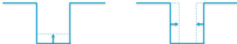
Figure 4.2: Schematic of different ways of supplying sediment, elevating the bed or narrowing the channel
