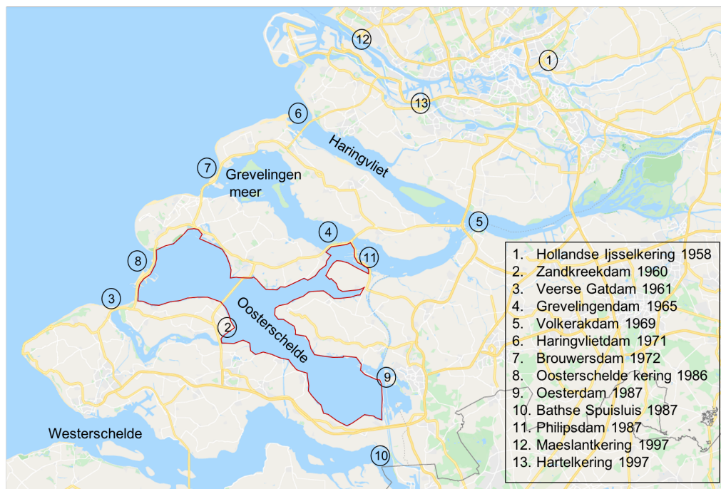
Figure 1.1: Overview of the Delta Works with the Eastern Scheldt domain indicated in red
