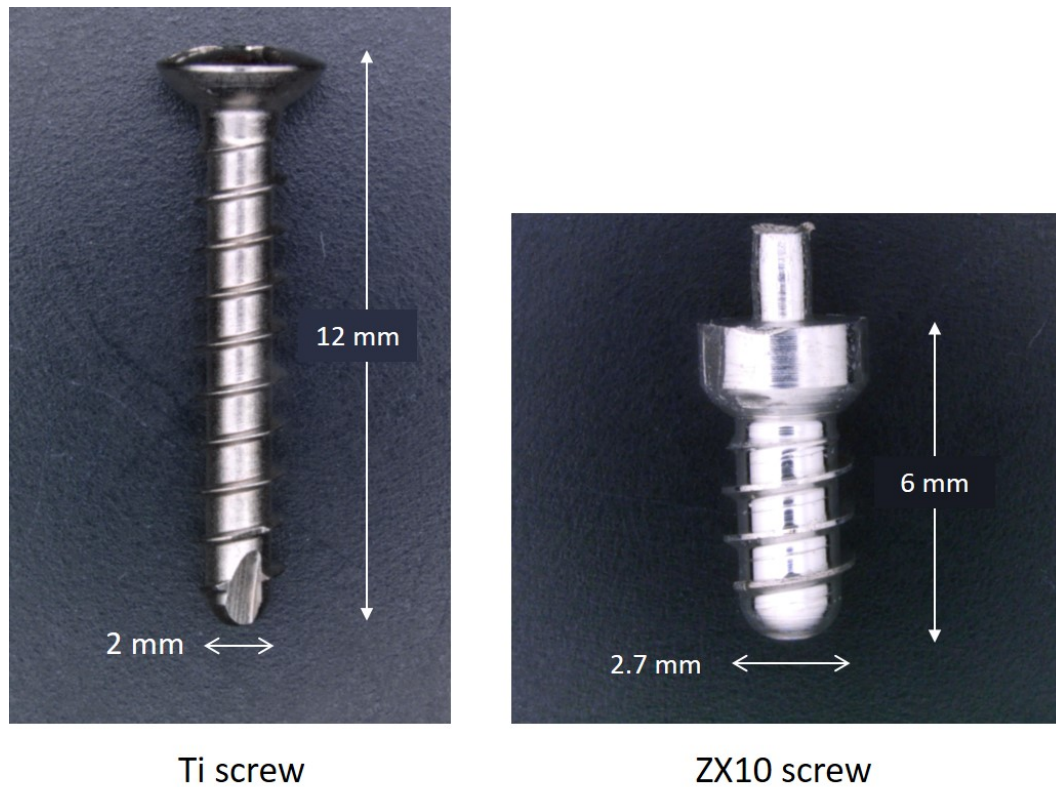
Figure 2.10: DePuy Synthes Ti screw and in house manufactured ZX10 screw used in the pull out experiment. Length of the screw and outer diameter are indicated.
