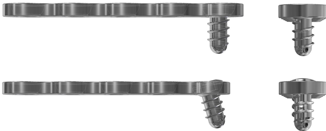
Figure 3.4: Assembly of the screw plate system showing orthogonal screw and screw inserted at 15°.
